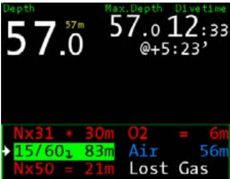
Gas list in dive mode: The Nx 50 has a too high ppO2 for the current depth.
